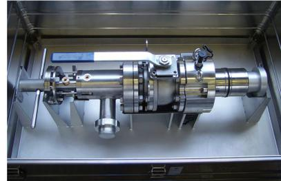
Tool to take a gas sample for radiolysis (developed for spent fuel containers type TN 17T)
